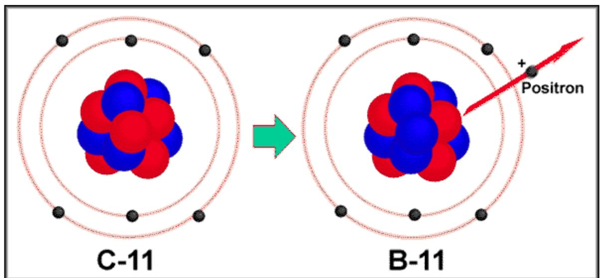
Positron Decay of Carbon-11 to Boron-11
